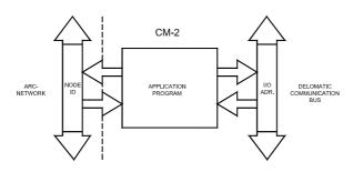
The CM also carries out mutual exchange of information and commands with the DELOMATIC modules installed in the DGU via the communication bus on the back plane.
