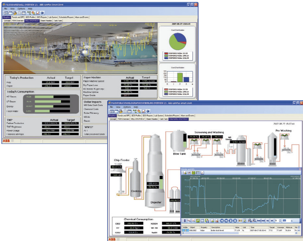
Figure 28. Using Smart Client, information from System 800xA for Harmony or connected third-party data sources is readily available on users' PCs and can be easily customized to allow access to the precise data needed to make better decisions
